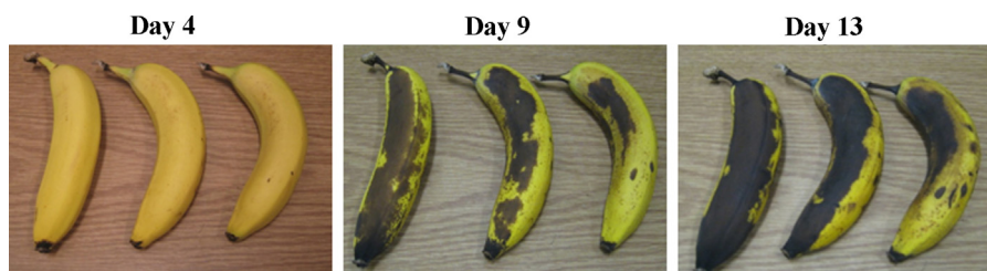
Fig. 3. Comparison of ripeness as function of time (from left to right) between uncoated control and bananas coated with 10 TL and 10 QL assemblies. Bananas were aged under ambient conditions (22 °C and 55% RH).
